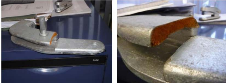
Figure C6.6: Proprietary brace connectors that failed during the February 22, 2011 Christchurch earthquake (M. Bruneau)
