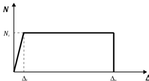
Figure C6.11: Force-displacement relationship for steel braces in tension
