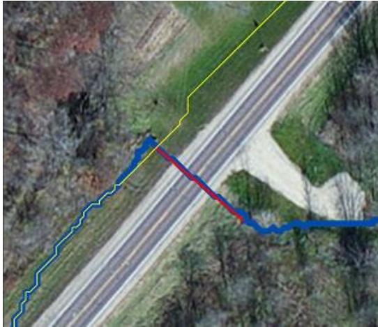
Figure 2. Unseen culvert resulted in LiDAR produced flow line in yellow parallel to roadway. Hydrologic cut line (red) allows actual road passage and represents actual flow (blue).
