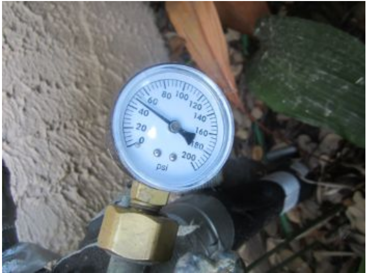
Water pressure at 50 PSI (acceptable)
