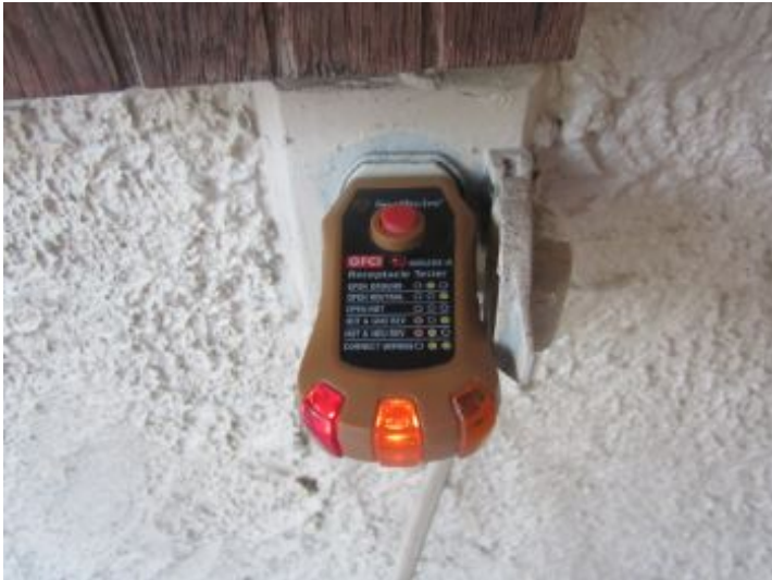
Hot and neutral reversed on exterior outlet
