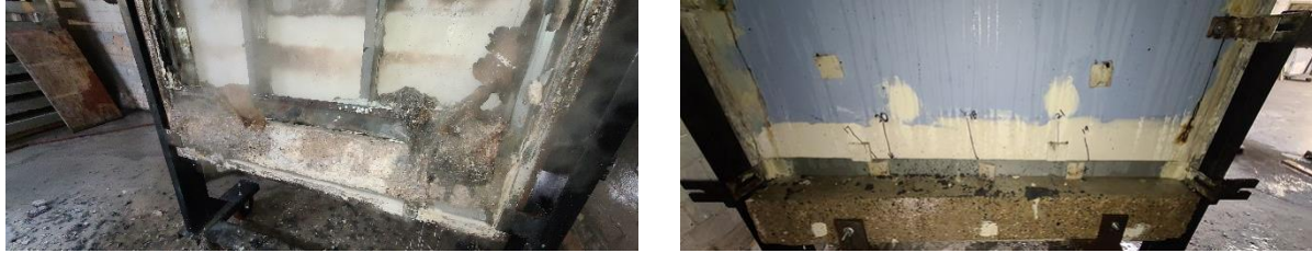
Figure 11: The assembly after hose stream exposure. The exposed side of assembly is on the left, and unexposed side on the right. The base reveal remained firmly in place on the unexposed side of the assembly throughout hose stream exposure. Observations show that there was no evidence for water passing through the Bottom of Wall firestop system.
