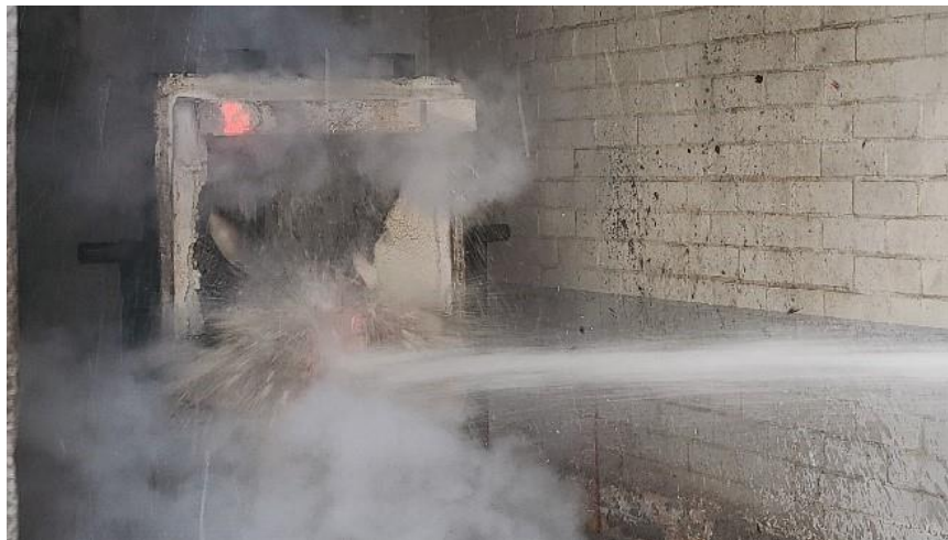
Figure 10: The test assembly was exposed to a 30-psi hose stream for 24-s per Table 19.1 in UL 2079.
