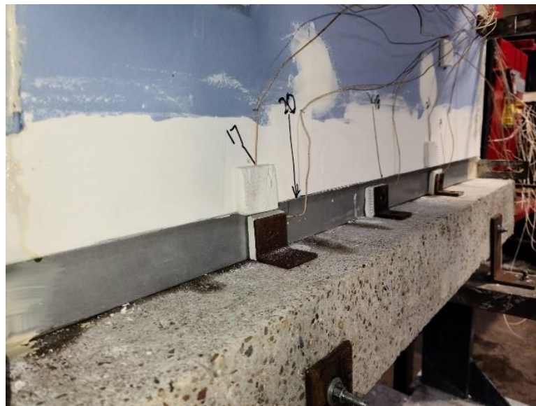
Figure 7: Moisture is visible at the base reveal and concrete interface, evidenced by the dark areas on the concrete shown in the image.
