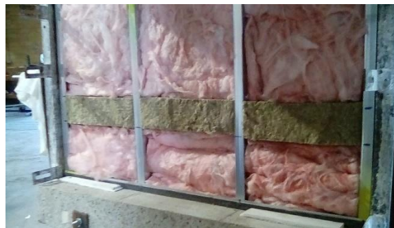
Figure 1: 1-1/4 inch leg floor runner (25-GA) and nom. 3-1/2 inch steel stud framing (20-GA, 16 inch OC) used to construct the wall. R19 fiberglass insulation fills the wall cavity.
